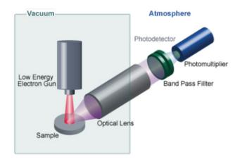
A dedicated Bremsstrahlung Isochromat Spectroscopy detector (BIS) is used with a selectable photon energy range up to 4.88 eV.
