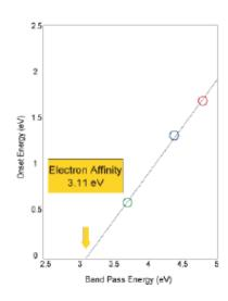
10 nm copper phthalocyanine thin film on ITO measured with 3 different band pass filters (BPF) allows for the calculation of the electron affinity by extrapolating to zero onset energy.
